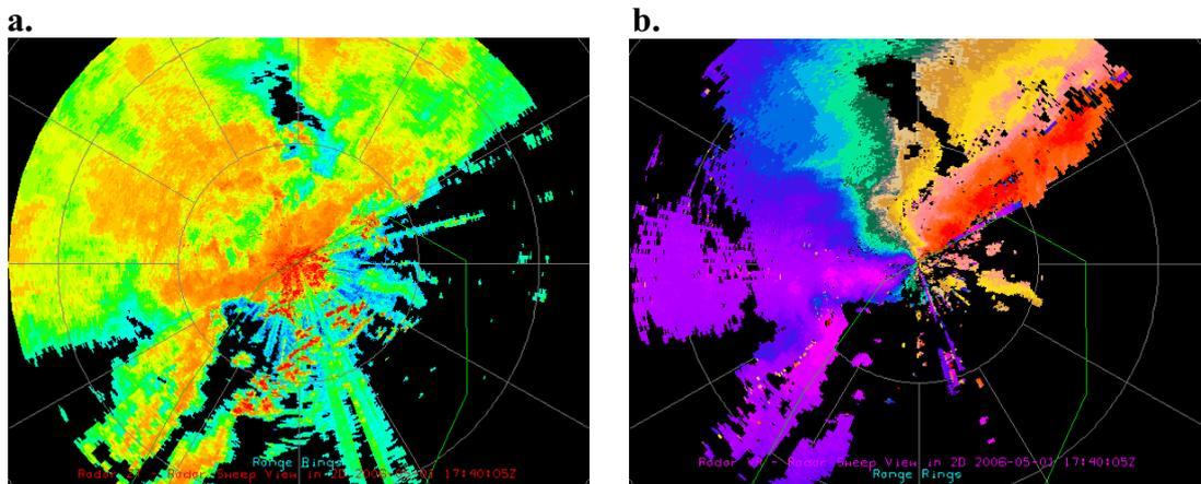
Fig 2. (a) Reflectivity and (b) Doppler velocity observed by the TIA Doppler weather radar at 0.5 elevation angle at 1740 UTC, May 1<sup>st</sup> 2006.
