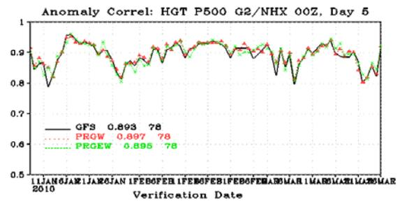
Fig. 2 Anomaly correlation for the Northern Hemisphere at 500 hPa after 5 days integration for cases from January to Mar 2010 with the operational GFS using sigma-pressure hybrid coordinate (GFS) and modified GFS using generalized hybrid coordinates (PRGW) and generalized hybrid coordinates with enthalpy as thermodynamic variable (PRGEW), with resolution of T382 and 64 layers.
