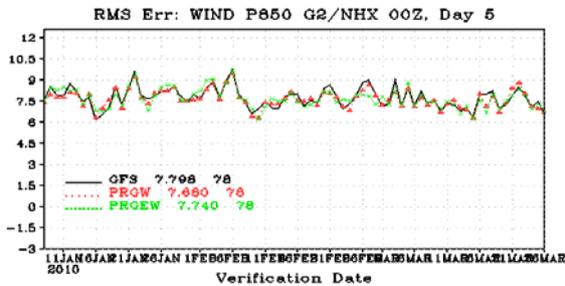
Fig. 6 Root Mean Square error of Northern Hemisphere vector wind at 850 hPa after 5-day integration for cases from January to March 2010 with operational GFS using sigma-pressure hybrid coordinate (GFS) and modified GFS using generalized hybrid coordinates (PRGW) and generalized hybrid coordinates with enthalpy as thermodynamic variable (PRGEW), with resolution of T382 and 64 layers.
