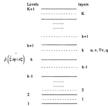
Fig.1 The vertical grid structure with layers and levels. Integers are used to index layers and levels; variables marked with hats are on levels and without hats are layers.
