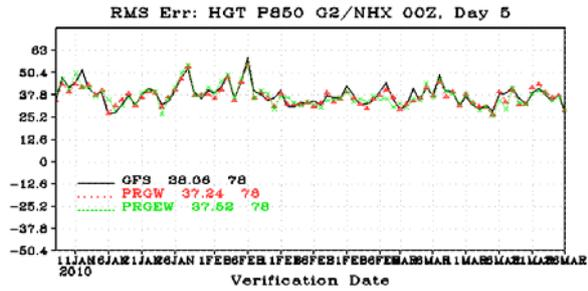
Fig. 5 Root Mean Square error of Northern Hemisphere geopotential height at 850 hPa after 5-day integration for cases from January to March 2010 with operational GFS using sigma-pressure hybrid coordinate (GFS) and modified GFS using generalized hybrid coordinates (PRGW) and generalized hybrid coordinates with enthalpy as thermodynamic variable (PRGEW), with resolution of T382 and 64 layers.
